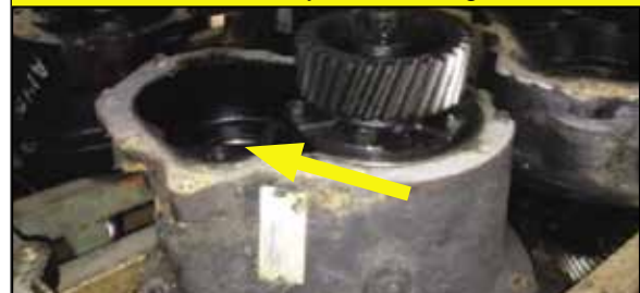
Carrier Core missing "Power Divider Cover"- Carriers were opened up and additional parts missing
