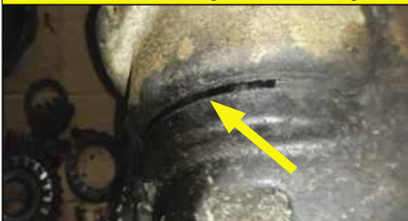
Failure crack through carrier housing
