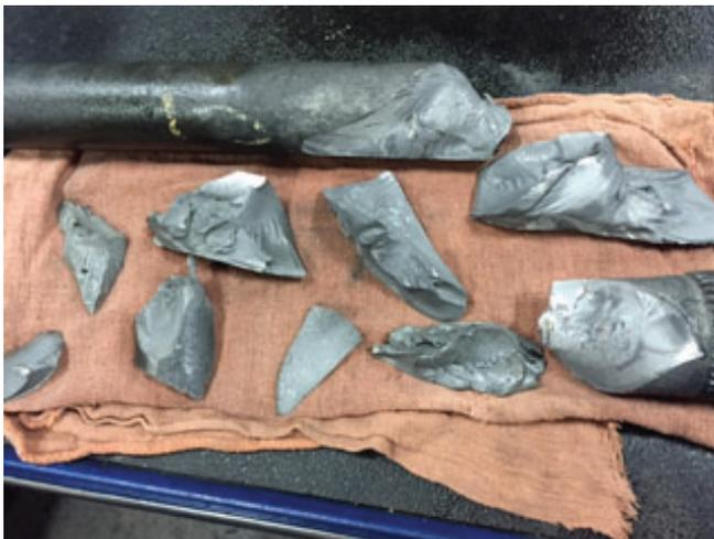
Axle Shaft - Torsional Shock
