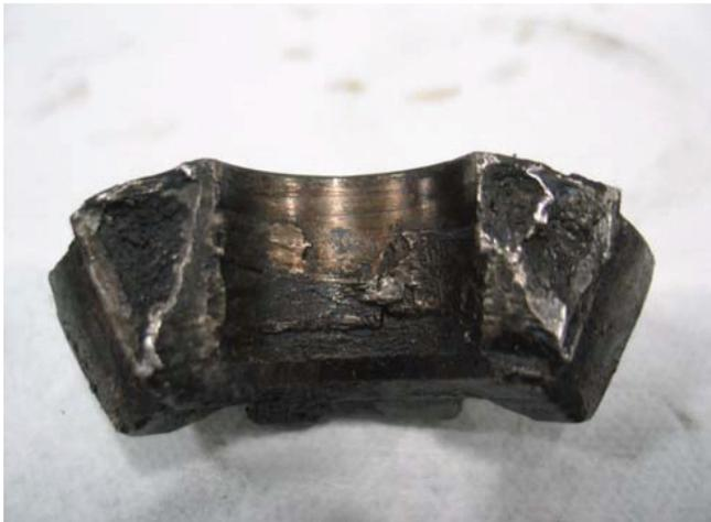
Thrust Washer to Input Shaft - Galling
