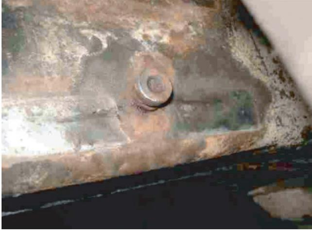
Over-torqued Clamping Hardware
