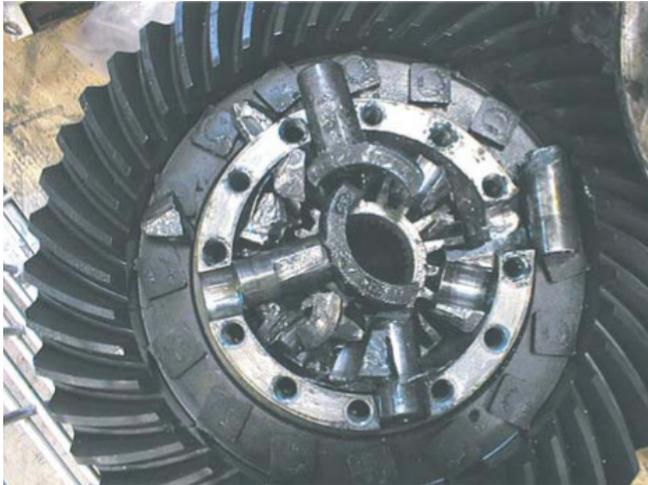
Wheel Differential - Side Pinion Shock
