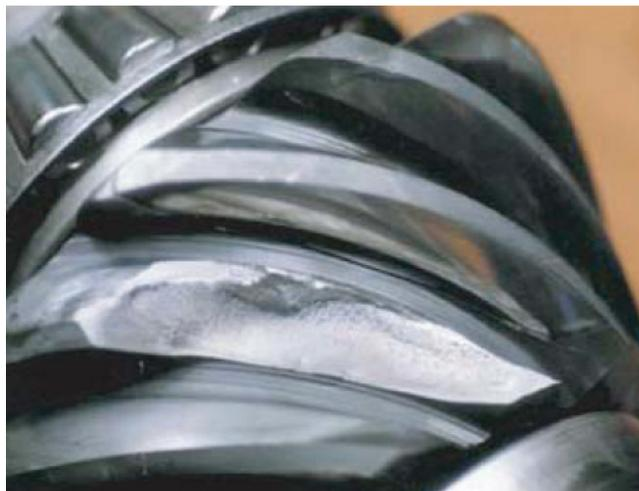
**General Description:** Shock damage occurs from overstressing the gear teeth or shaft beyond the strength of the material. The failure could be immediate (from a sudden shock) or progressive (cracking of the teeth or shaft surface following the initial shock).
