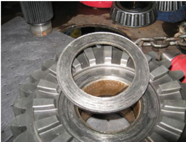
Power Divider Spinout - Stub End Galling
