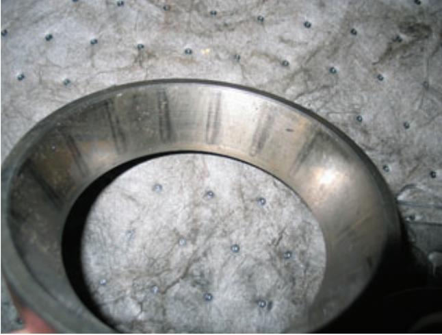
Bearing Cone - Spalling
