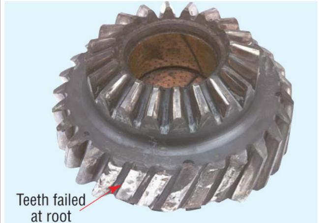
Input Shaft - Torsional Shock
