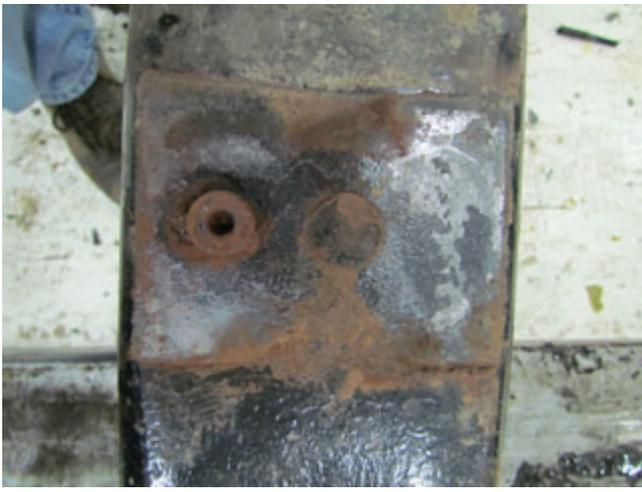
**General Description:** Sufficient clamp load at the spring pad area is important to keep the joint tight. Loose clamping or overtorqued clamping hardware resulting in cracks in the drive axle housing.
