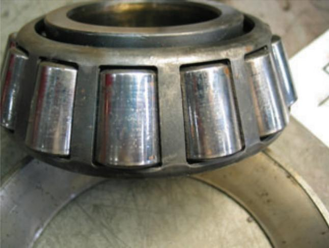
Bearing - Lack of Lubrication
