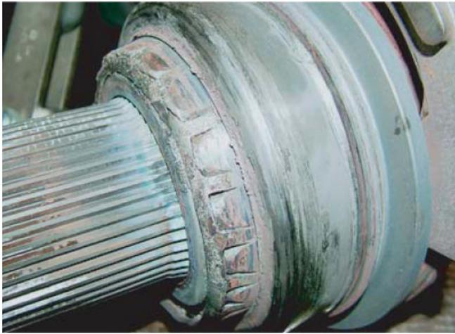
Output Side Gear Bearing - Low Lube
