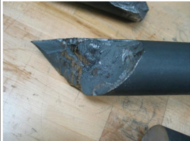
Axle Shaft - Torsional Shock
