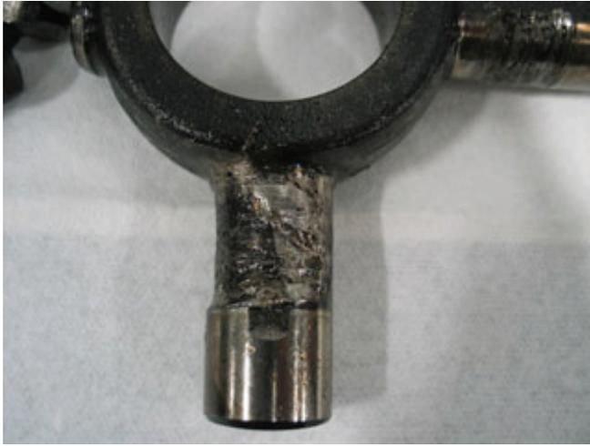
Wheel Differential Side Pinion - Spinout Galling
