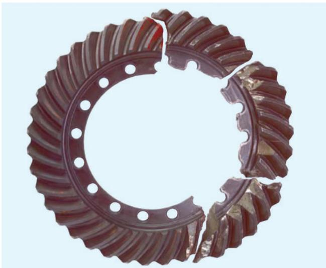
Ring Gear - Coast Side Shock Failure
