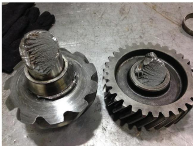
Drive Pinion - Tooth Shock Load Failure
