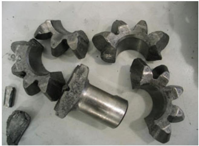
**General Description:** Shock damage occurs from overstressing the gear teeth or spider beyond the strength of the material. The failure can be immediate (as from a sudden shock) or progressive (as cracking of the teeth or shaft surface following the initial shock).
