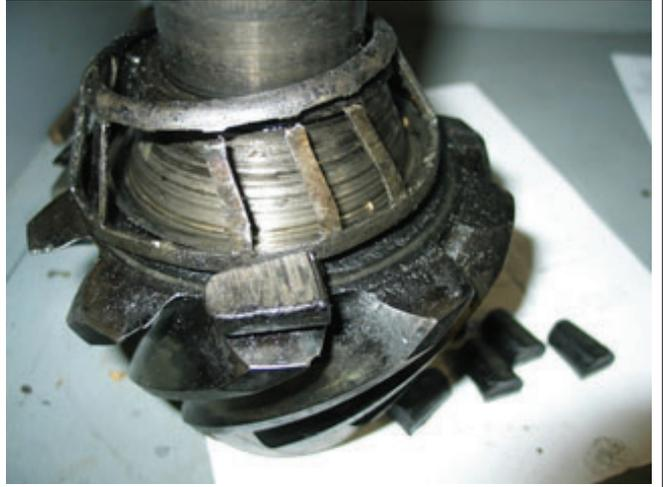
Bearing Cone - Spalling - Water Damage
