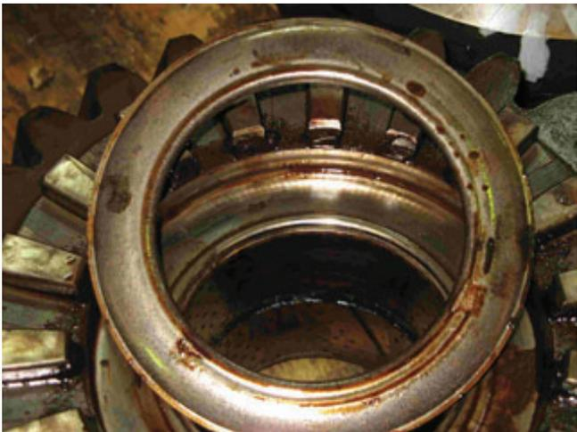
Helical Side Gear Bushing - Water Damage
