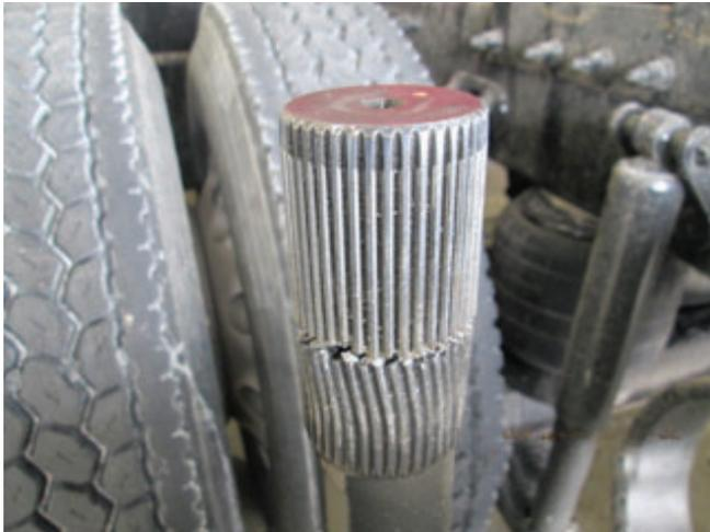
Axle Shaft - Torsional Shock
