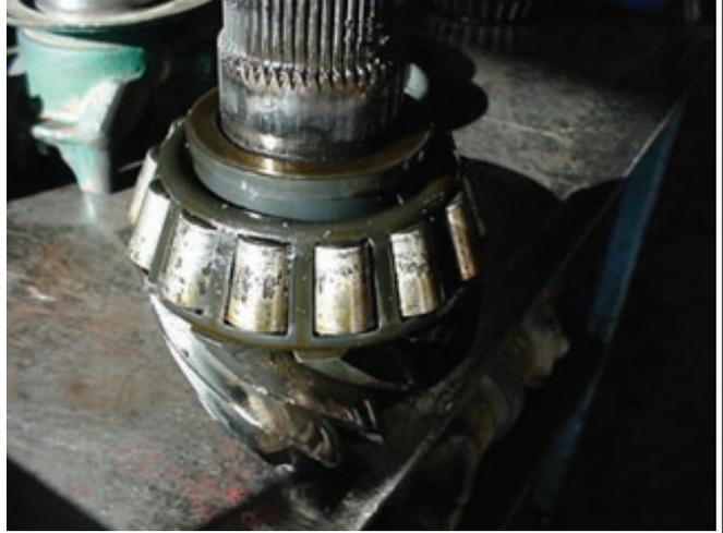
Bearing - Excessive Bearing Preload - Heat
