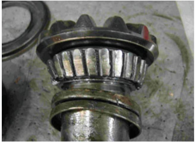
Helical Thrust Washer - Water Damage
