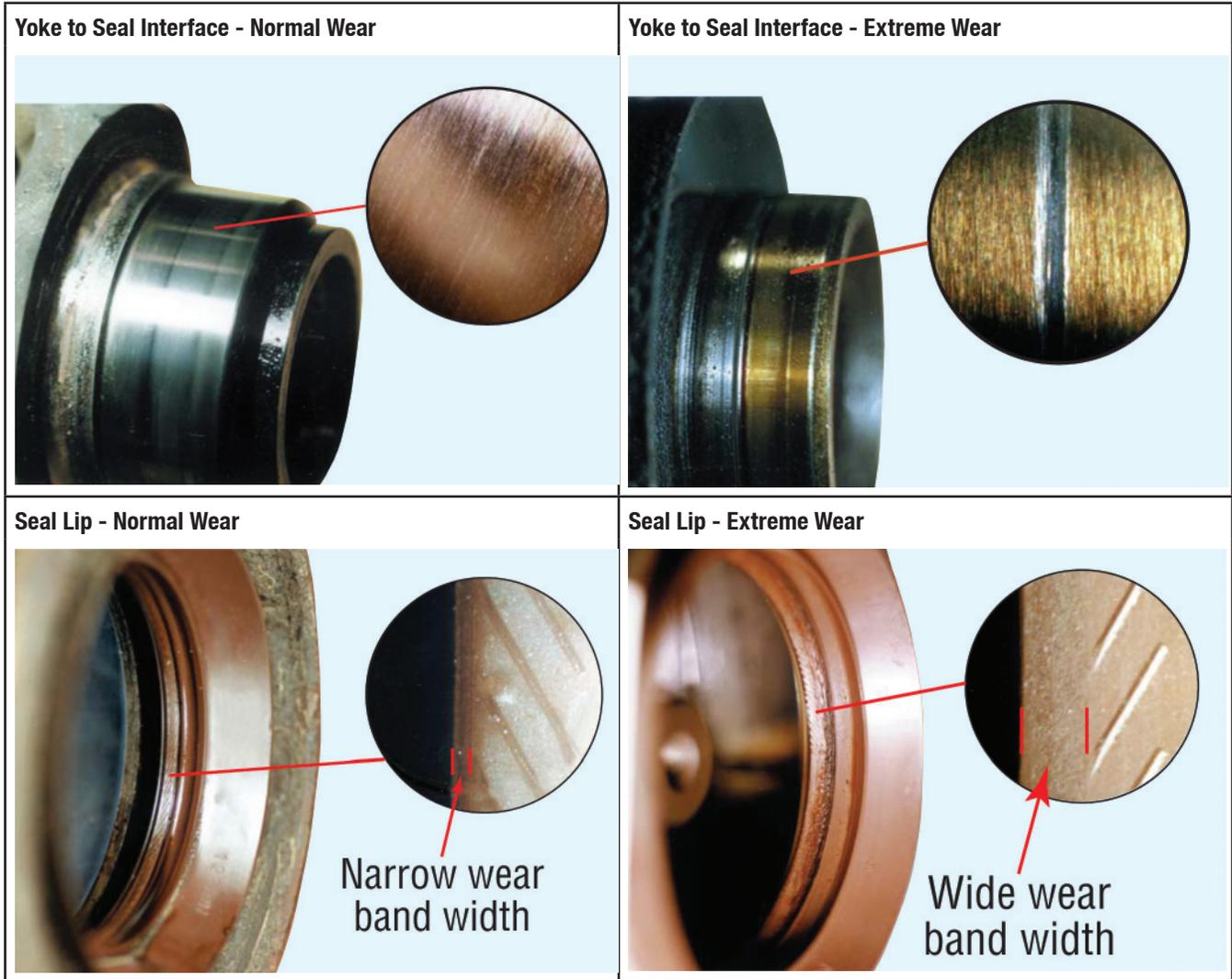
**General Description:** Yokes and seals will have a shortened wear life if not installed correctly. A worn yoke or seal will also allow contaminants into axle lubricants.
