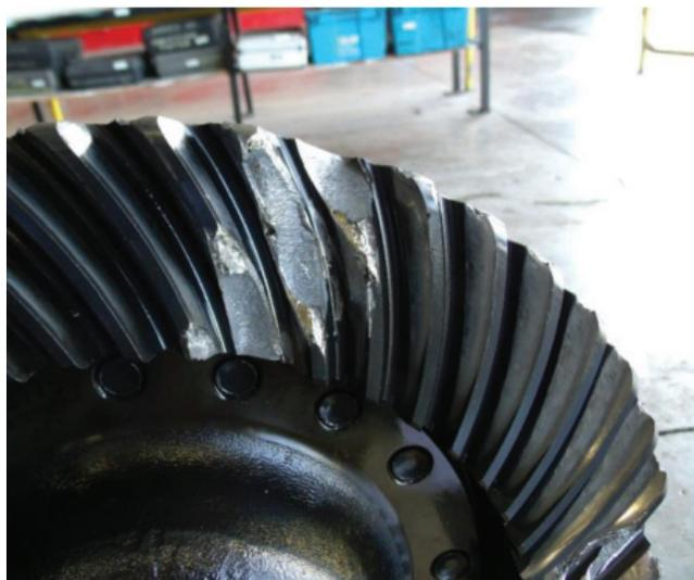
Ring Gear - Coast Side Shock Failure
