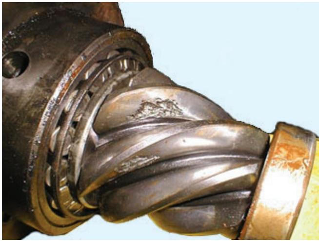
Pinion Spline - Water Damage - Wear
