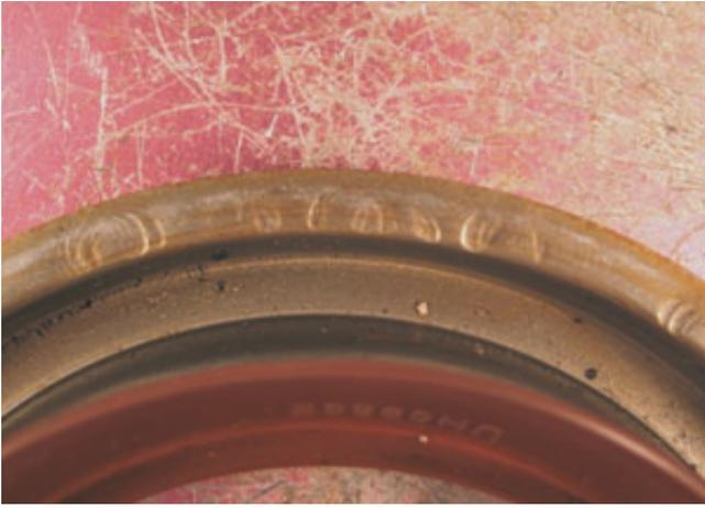
Dirt Between Seal and Bearing Cage
