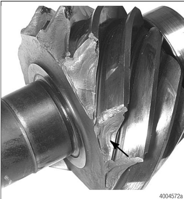
**TEETH BROKEN DUE TO FATIGUE AT HEEL END**
