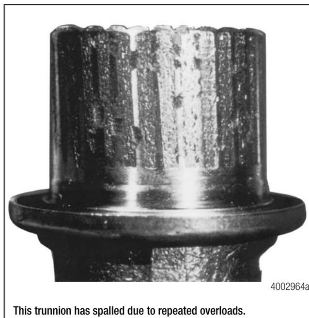
This trunnion has spalled due to repeated overloads.
