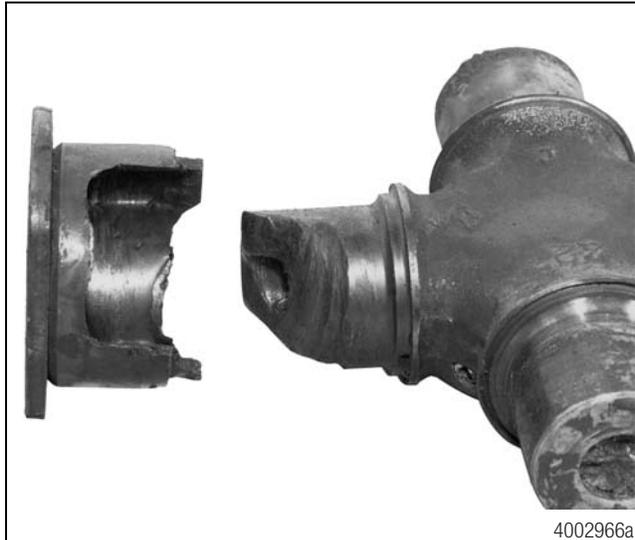
This universal joint shows the damage that can happen from lack of lubricant. The friction and heat created by the lack of lubricant caused the universal joint trunnion to wear through the side of its roller bearing cap.
