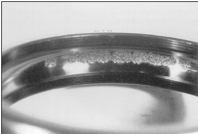
Figure 47 — Flaking on One Side of the Race Surface
