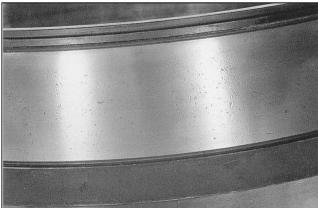
Figure 49 — Inner Race Surface Indentations
