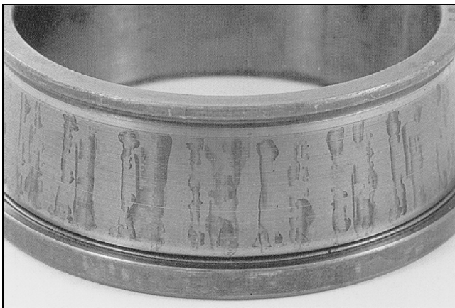
Figure 32 — Tapered Roller Bearing Rust on Raceway
