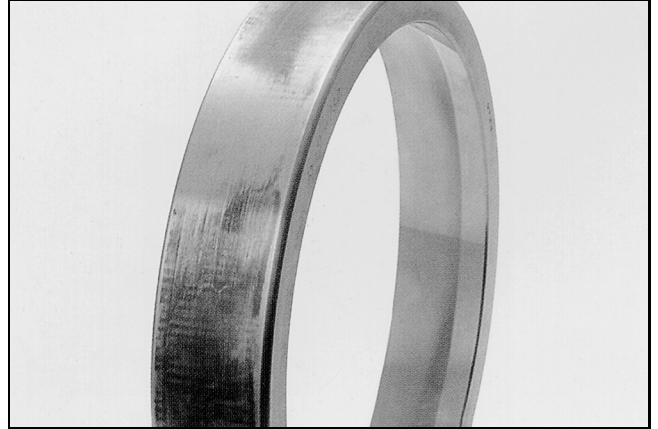
Figure 53 — Fretting and Fretting Corrosion
