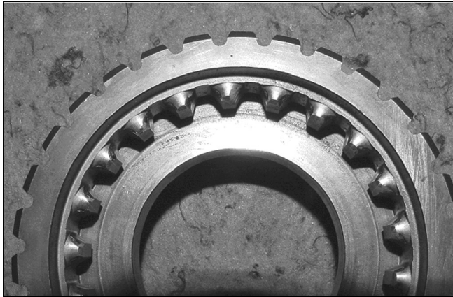
Figure 98 — Typical Warranty Returned T310M Low Range Hub Gear Synchronizer Teeth Failure
