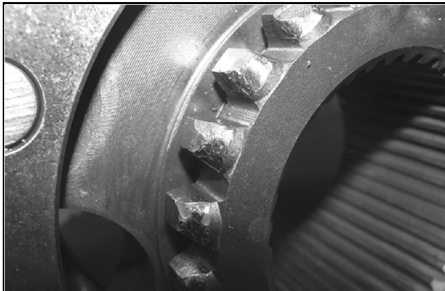
Figure 95 — Typical T310 High Range Synchronizer Clutch Teeth Failure
