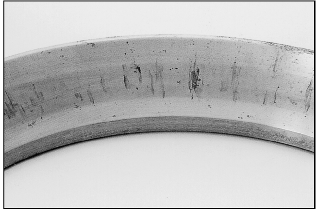
Figure 51 — Rust and Corrosion
