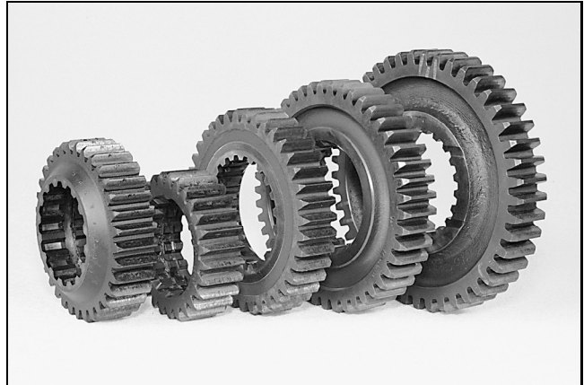
Figure 76 — Inadequate Lube/Lack of Lubrication
