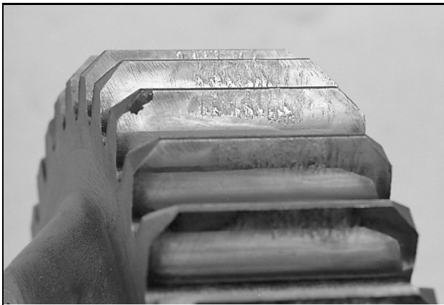
Figure 80 — Damaged Tooth Flank
