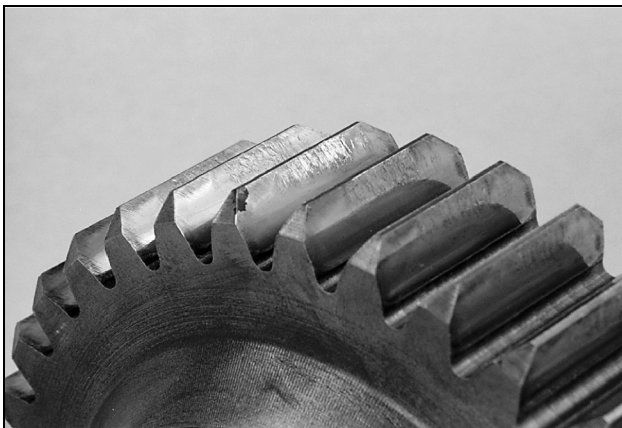
Figure 79 — Damaged Tooth Flank
