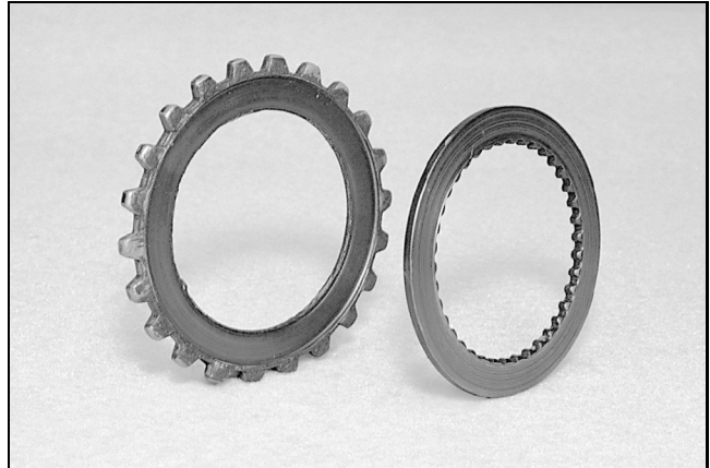
Figure 55 — Thrust Washer Wear
