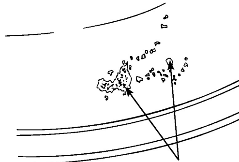
Figure 42 — Tapered Roller Bearing Flaking/Spalling
