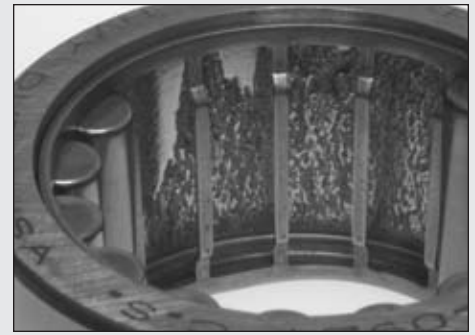
Fig. 38. The housing bore was machined with an improper taper, causing the uneven load distribution and GSC spalling in this cylindrical roller bearing outer ring.
