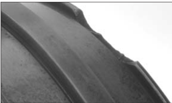
Fig. 40. This spherical roller bearing inner race depicts a fractured small rib caused by the use of improper installation tools.
