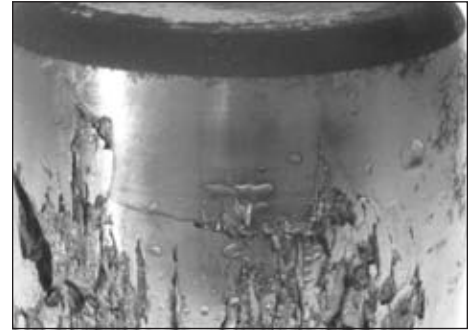
Fig. 25. Heavy spalling and fracturing from high loads on this spherical roller bearing.
