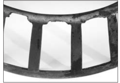
Fig. 34. Heavy wear in the small end of the cage pockets is typical of excessive endplay.
