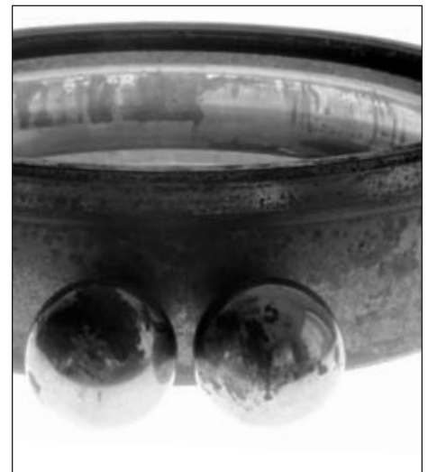
Fig. 16. This ball bearing outer race also depicts etching and corrosion.
