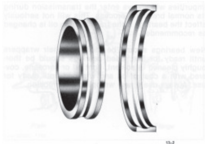
Ball path pattern caused by out-of-round squeeze
