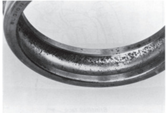
Burnt and spalled bearing 13-3
