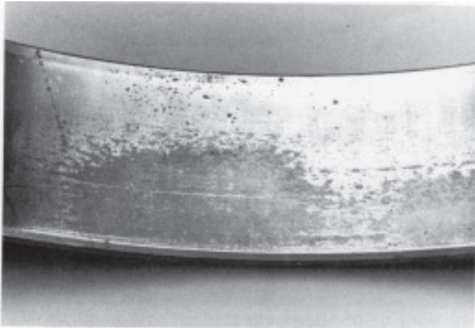
Bearing race "flaking" 13-1
