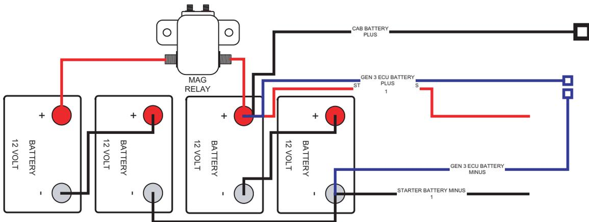
**TWO BATTERY BANKS - TWO BATTERIES PER BANK WITH DISCONNECT**
