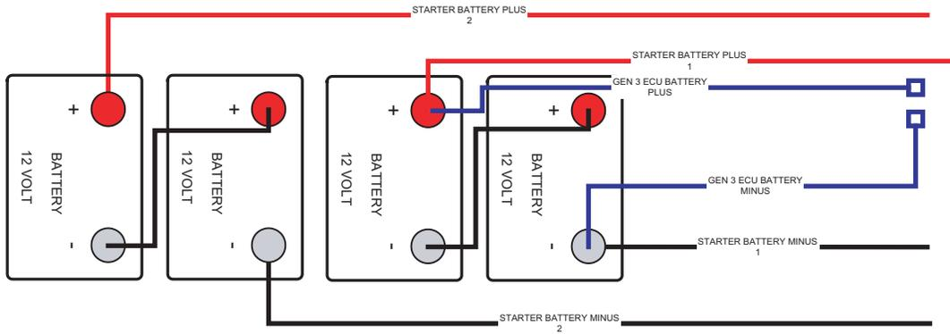
**TWO BATTERY BANKS - TWO BATTERIES IN SERIES PER BANK - DUAL JUMPERS TO STARTER**
