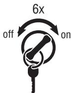
**Note:** If the codes have been successfully cleared, the Service light will come on and stay on for five seconds. The gear display will show 25 (no codes).
