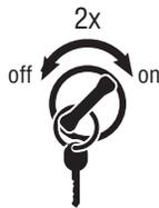
5. To Retrieve Inactive Codes: Turn key on. Turn the key off and on 4 times within five seconds ending with the key in the on position. After 5 seconds, the Service light begins flashing two-digit fault codes. If no faults are active, the service light will flash code 25 (no codes).
