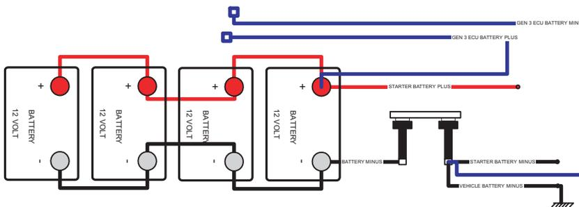
**TWO BATTERY BANKS - BATTERY NEGATIVE DISCONNECT SWITCH**
