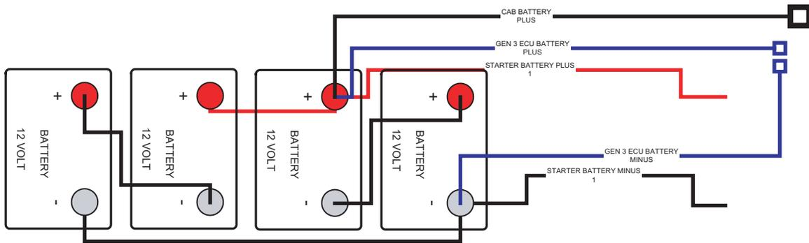
**ONE BATTERY BANK - FOUR BATTERIES - ONE CABLE PAIR TO STARTER**
