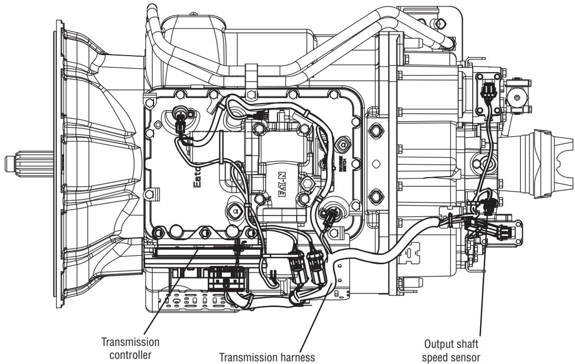
**Note:** If troubleshooting an UltraShift *PLUS* model transmission's Output Shaft Speed Sensor, which is a directional sensor, go to Step E; otherwise, start at Step A.
