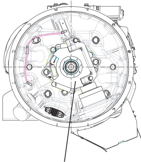
Low Capacity Inertia Brake
