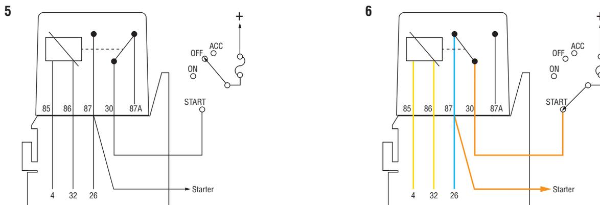
**Start Enable Relay Circuit States (Normally Open)**
