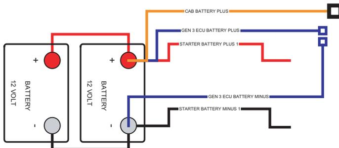
**ONE BATTERY BANK - TWO BATTERIES**
