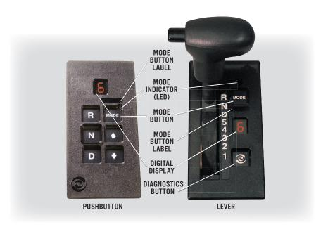
Vehicle manufacturers may choose different types of shift selectors for their vehicles. The shift selector in your Allison-equipped vehicle will be similar to one of the pushbutton or lever styles as shown above.
